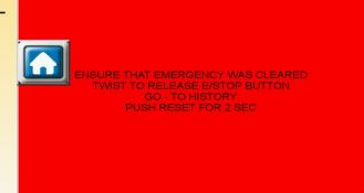
This means that the Emergency stop push button was pressed. MAKE SHURE !!! that the emergency situation has been cleared. Twist to reset the e/stop button.
