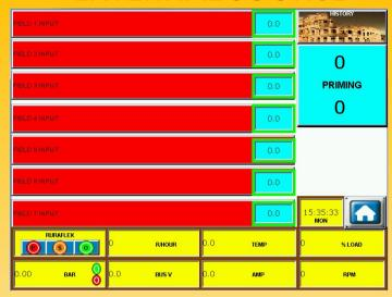
17: External source – This was developed to accommodate irrigation computers. Seven Fields / pressures can be activated via the digital inputs (see electrical drawing). Please note that the 24vdc source provided at terminal 3 (white wire) must be used and not an external power supply.
